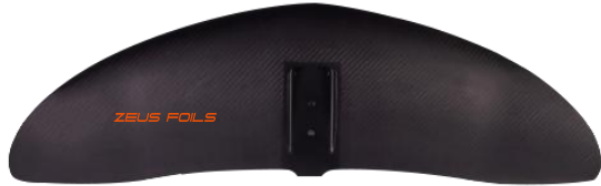
ZF-ONS 820 Front wing Area :1443 sqcm Front wing size:820 * 223mm volume: 2657cm 3
